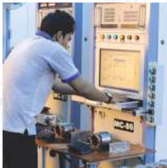
Surge Impedance Test
