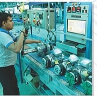
Brake Motor Testing
