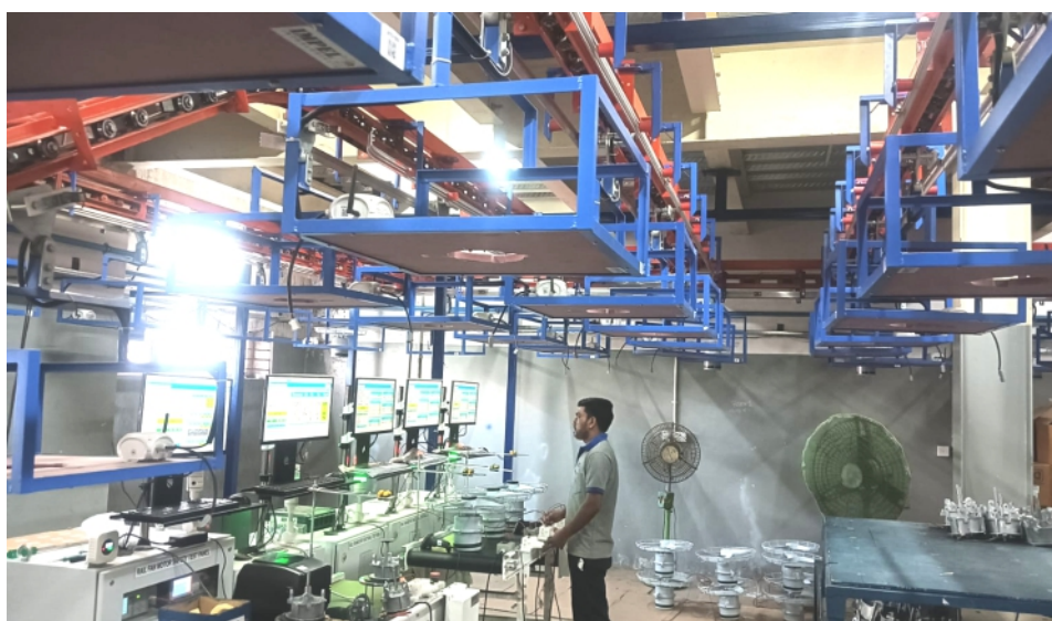
Testing Conveyor for BLDC Fans
