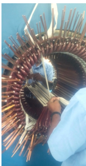
Coil insertion in stator
